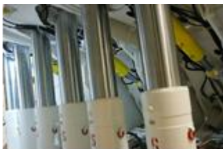
Hydraulic props (legs) covered with DURACHROM unique protective ecological coatings
