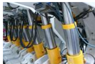
Hydraulic props (legs) covered with DURACHROM unique protective ecological coatings
