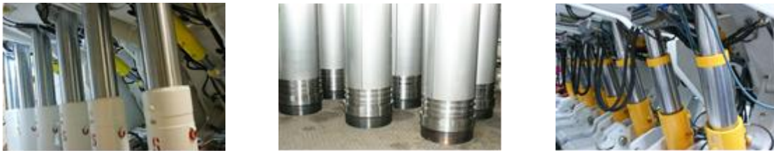
HYDRAULIC PROPS COATED WITH A LAYER OF UNIQUE DURACHROM PROTECTIVE COATING
